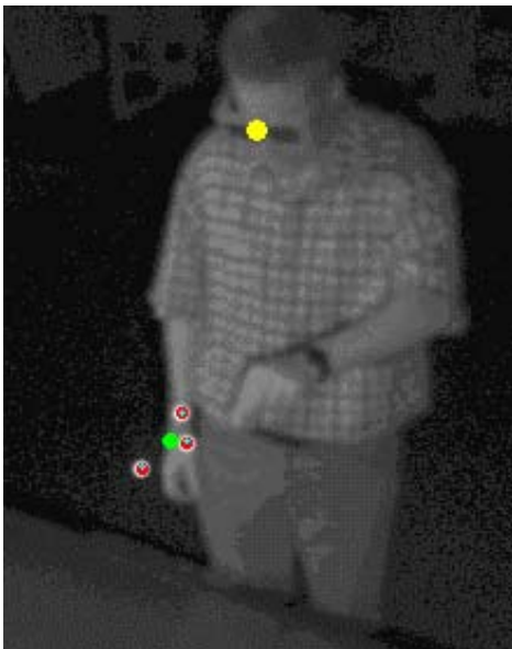
Figure 1: View from one of the cameras with infrared filter. Three passive markers for the hand device (green dot) and one passive marker for the head (yellow dot) are tracked and superimposed with segmentation results (red dots) on the camera image.
